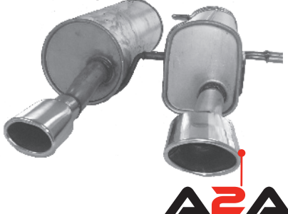
Stainless Steel Tail Pipe - not mild steel chrome plated
