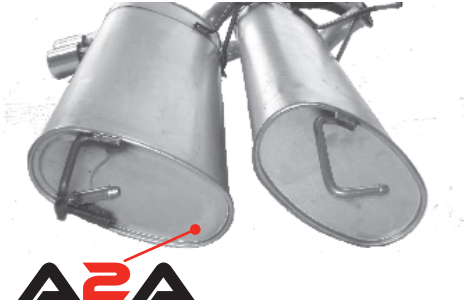
Dished End Plate - for sound reduction
